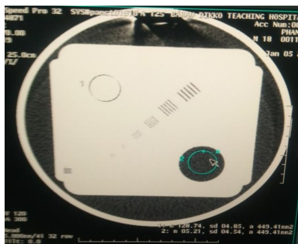
Figure V: Scanner I CT QC image for low contrast resolution
